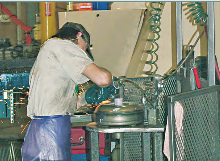
Once a core enters the remanufacturing process, it is cut open and disassembled.
